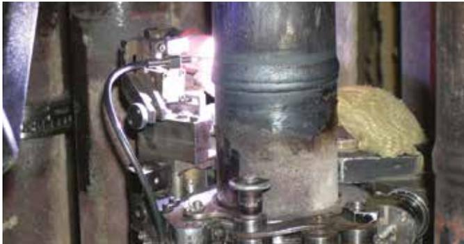
*Orbital tube welding*
