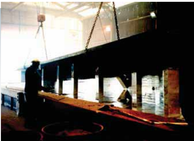
Progressive dipping - galvanizing oversized pieces
