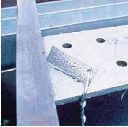
Figure 30: Tag for identification affixed with a minimum #9 gauge steel wire
