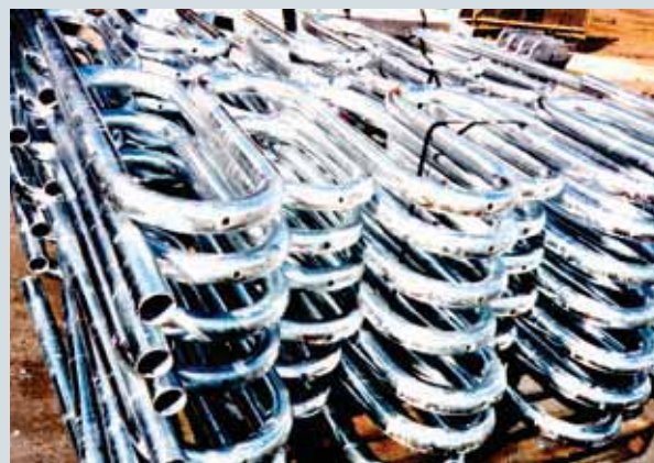
Hot-dip galvanizing cold-worked steel is very successful when following suggested guidelines
