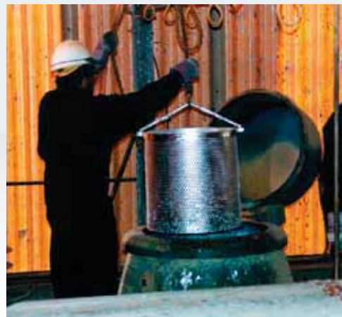
A perforated basket filled with bolts is placed in a centrifuge to spin off excess zinc
