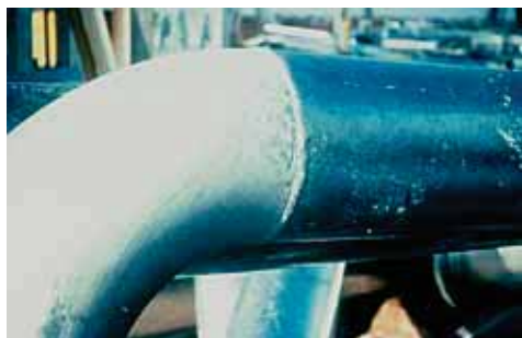
Varying steel chemistries create visually different coatings, as illustrated by this pipe assembly
