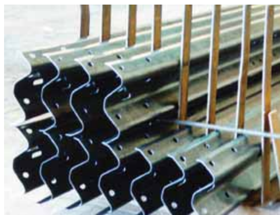
Galvanized guard rail stored with wood spacers to avoid wet storage stain
