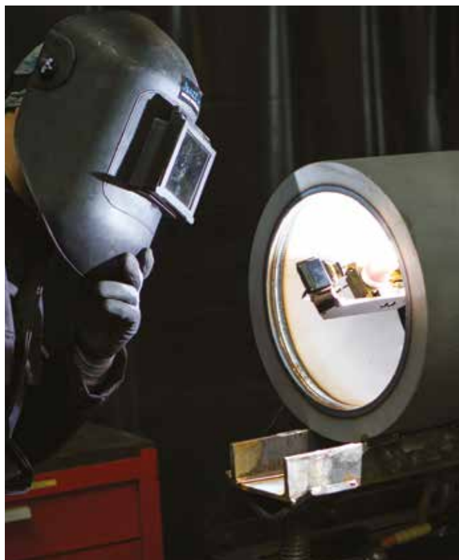
AZZWSI offers a unique, fully automated repair solution for the Nozzle ID covering a range from 2 to 24 inches
