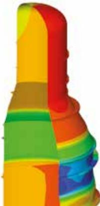
Shaded plot of vacuum column predicted diametric shrinkage
