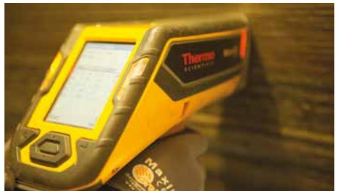
PMI/FN inspection using XRF
