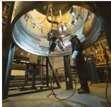
Mock-up for automatic weld overlay
