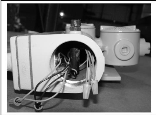
6. Remove the red LED indicator assembly from the housing.
