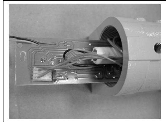
11. Remove the circuit board from the housing.
