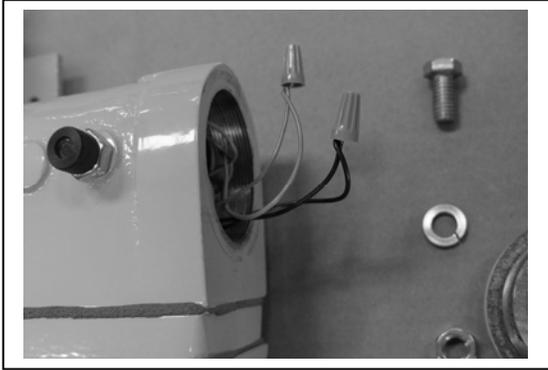
3. Pull the wires out on the side of the housing.
